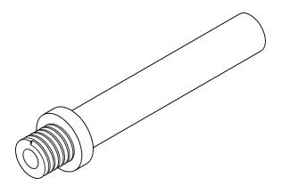
Post is drilled thru 1/4" diameter. Provides clearance for drill bit and exit for chips.
