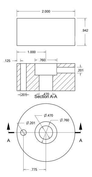
Both .201 holes are tapped 1/4-20. One for the lifting rod and one for the operating handle/weight rod. Center hole and counterbore is for a metric shoulder bolt. This bolt has 10mm threads. Optional to turn your own shoulder bolt.
