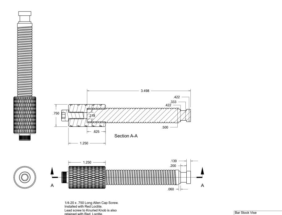
Lead screw to Knurled Knob is also retained with Red Loctite.
