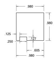
The center .376 hole and counterbore may be eliminated if not using the fixed jaw spacer for the Bar Stock Version.
