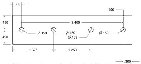
Total of 4 0.159 holes. The two on the outside are threaded from the front for the replaceable jaw faces. The two in the center are threaded from the back for an accessory part stop. Drawings for the part shop will be in an additional assembly drawing package.
