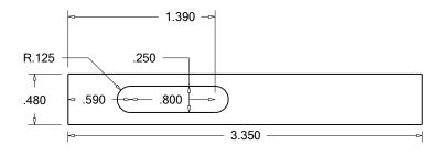
Swing Arm 1018 Steel .5 x 1.125 x 3.35 inches Blank. Tap 3 Places 10-32 for tool tool bit clamp. Slot .312 for 1/4 or 3/16 tool bit ground for threading. Bottom slot should be slip fit for key. Adjust as necessary. Best way is to file the key.
