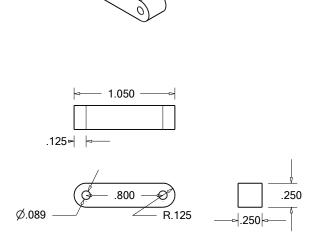
Key..Made From Key Stock or 1/4 square bar 1018. Drill two places 0.089 for tapping with 4-40 tap. Using file buttons file the ends round. Using emery cloth or wet/dry 220 grit pager to reduce sides for a slip fit into the slot of the Swing Arm. File or Mill the top surface for a clear fit into the Swing Arm
