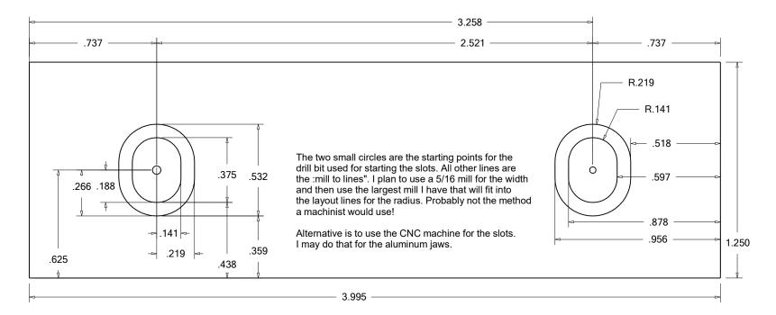
Main purpose of this drawing is for manual layout of slot dimensions. I use this for visual confirmation while milling just in case my digital readouts hickup.. Sometimes they do!
