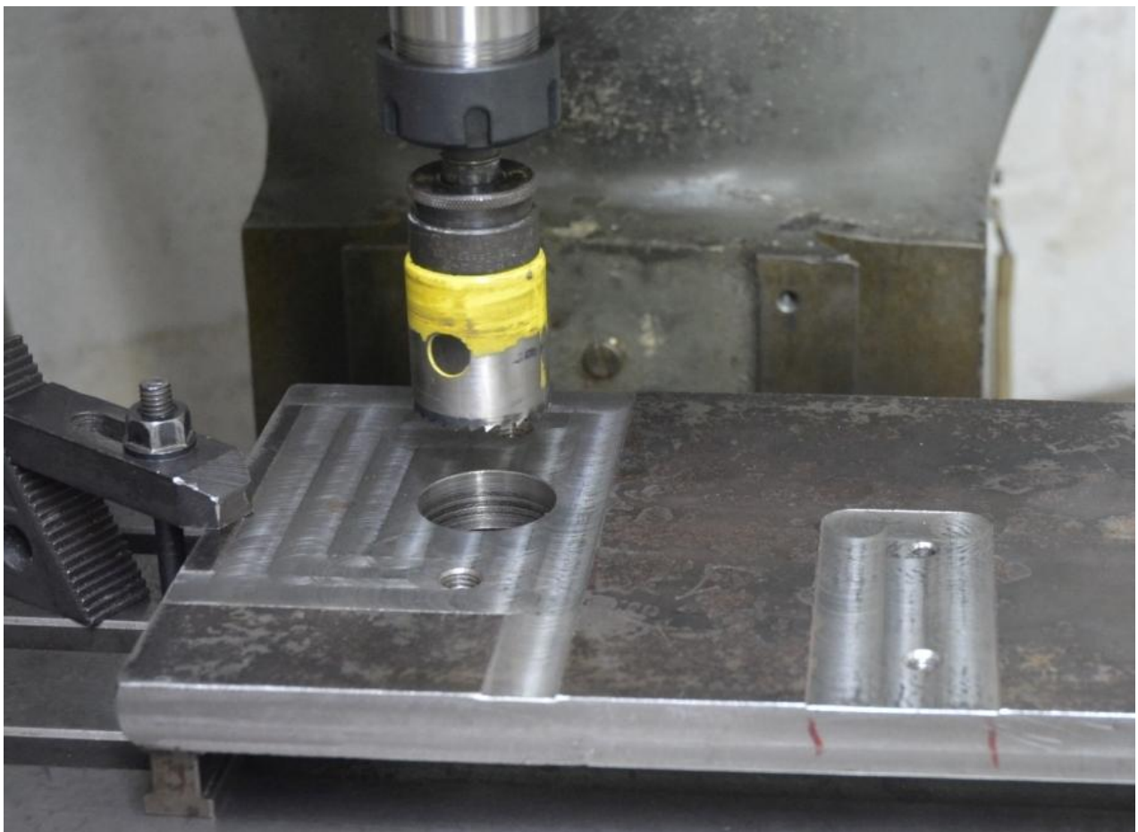
In this photo of the hole saw, and the boring head in the next photo, we can see one of the original tapped holes in the column surface near the top of the dovetail slides, as mentioned previously. These tapped holes are used to hold the plate in place.
