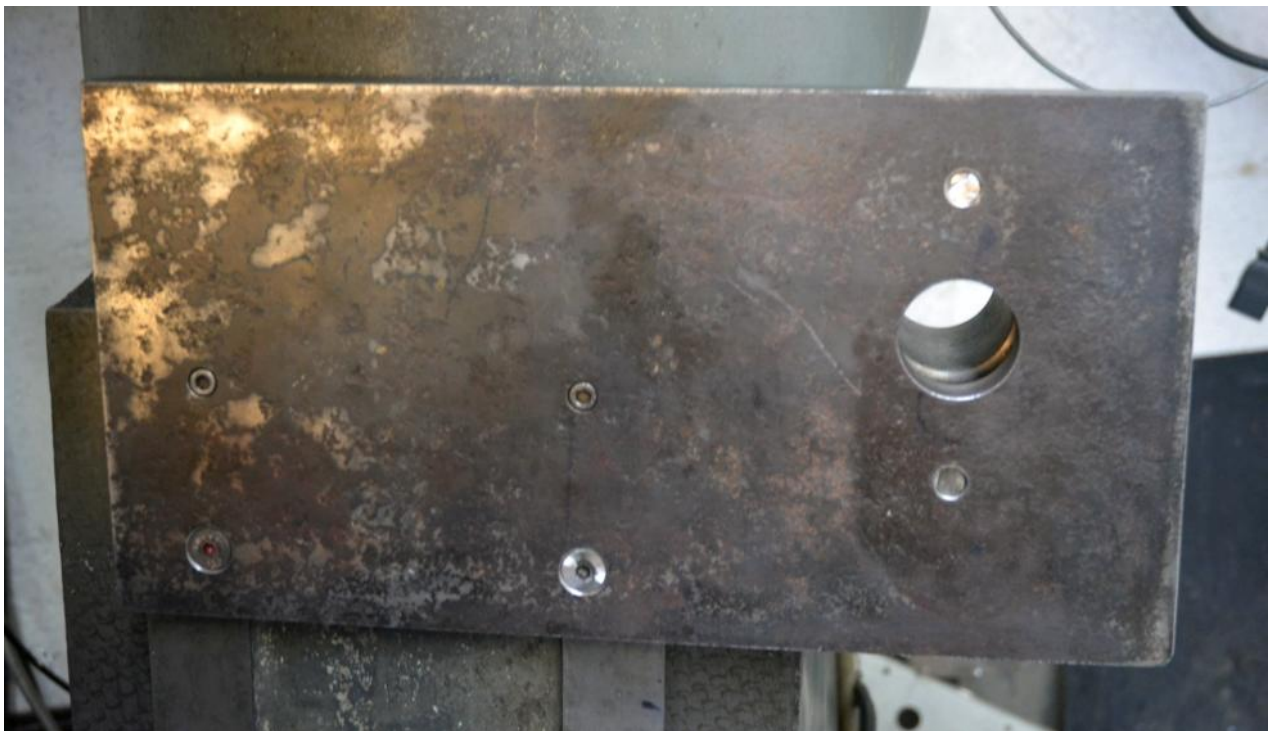
Here is the plate mounted to the mill column after being machined on the back side. The next photos show the spindle mounted in its bearings.
